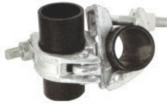
ISFC - SCBT SWIVEL COUPLER BRITISH TYPE FOR TUBE OD 48.3mm (EN-74 / BS 1139)
